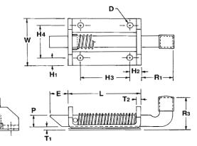
This rugged slam latch is ideal for applications that require a quick and effortless locking mechanism, such as truck and trailer doors, drawers and tailgates, as well as medical and farm equipment.
