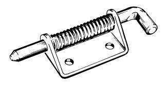
The Paneloc heavy-duty 720 Series spring latch features a 1/2" pin diameter. This large, rugged latch is available in steel or stainless steel and has a closed knuckle for added durability and strength. It is ideally suited for truck bodies, utility vehicles, horse trailers and more. The offset body design provides more flexibility with placement on tight applications.
