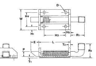
This rugged slam latch is ideal for applications that require a quick and effortless locking mechanism, such as truck and trailer doors, drawers and tailgates, as well as medical and farm equipment.
