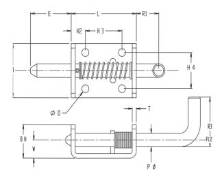
The Paneloc 785 Series Spring Latch features a 3/8" pin with a holdback.
