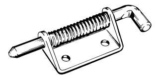
The Paneloc heavy-duty 719 Series spring latch features a 3/8" pin diameter. This large, rugged latch is available in steel or stainless steel and has a closed knuckle for added durability and strength. It is ideally suited for truck bodies, utility vehicles, horse trailers and more. The offset body design provides more flexibility with placement on tight applications.
