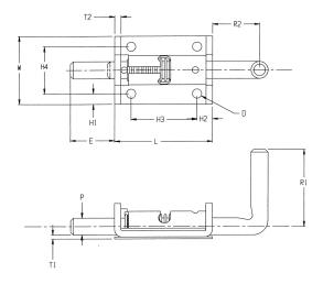
Paneloc heavy-duty spring latches are available in 3/8" and 1/2" pin diameters. These large, rugged latches are available in steel or stainless steel and have a closed knuckle for added durability and strength.
