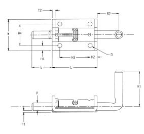
Paneloc heavy-duty spring latches are available in 3/8" and 1/2" pin diameters. These large, rugged latches are available in steel or stainless steel and have a closed knuckle for added durability and strength..
