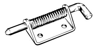
The Paneloc heavy-duty 719-720 Series spring latches are available in 3/8" and 1/2" pin diameters, respectively. These large, rugged latches are available in steel or stainless steel and have a closed knuckle for added durability and strength. They are ideally suited for truck bodies, utility vehicles, horse trailers and more. The offset body design provides more flexibility with placement on tight applications.
